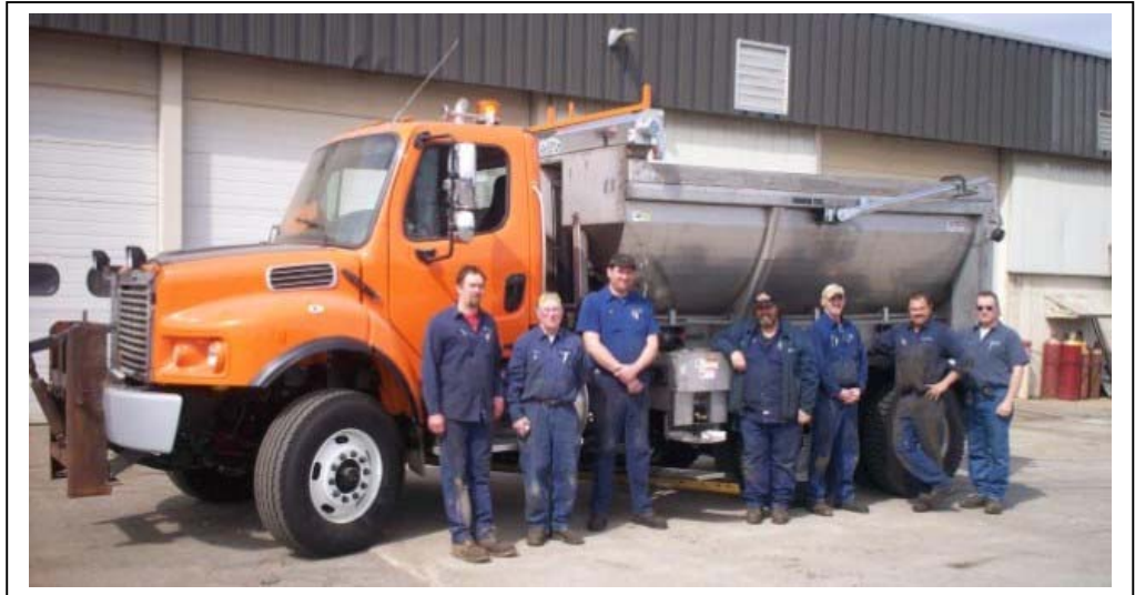
Photo of Staff in front of new tandem axle live bottom stainless steel dump truck with a mid mounted material cross conveyor being assembled. Pictured left to right: Rob Hahn, Clare Piepkow, Jay Phelps, Jeff Switzenberg, Chuck Barrett, Don Warvel, Duane Yerks. Not pictured in this photo is Jim White.
